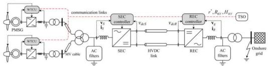
Fig. 1. Generic layout of an offshore WT connected through a VSC-based HVDC transmission link.
