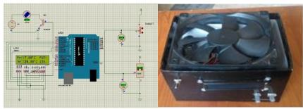
Figure 5. Design of project in Proteus and implementation in real-time
