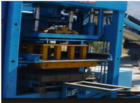
Figure 2. Concrete locked parquet stone production
