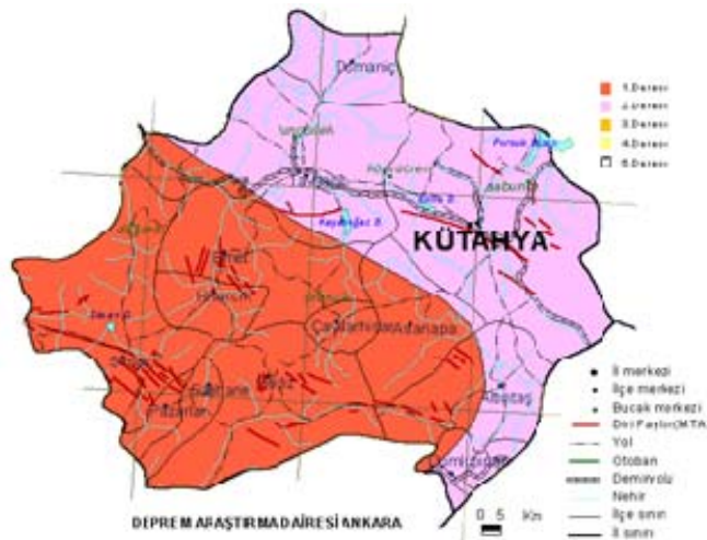
Figure 6 .Kutahya regional earthquake map, Republic of Turkey Prime Ministry Disaster and Emergency Management Presidency Directorate General of Earthquake [4].
